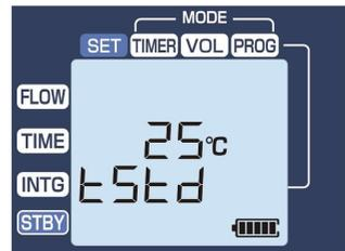
(When the flow rate conversion temperature is 25°C)
